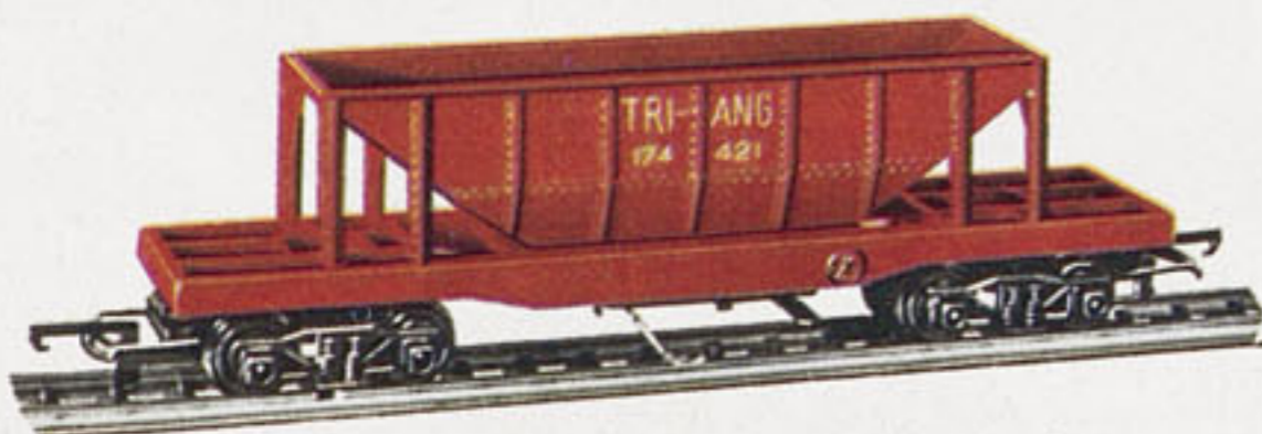
R.111 Hopper Car. With gravity unloading mechanism. 5\frac{1}{4} " (14.4 cms.) long.
